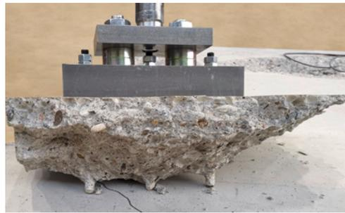
Concrete failure cone of a group of 3 anchors close to a concrete edge
