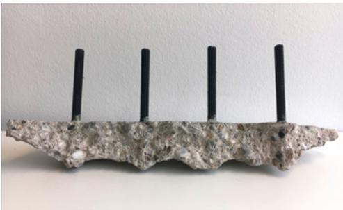
Typical breakout body of an anchor group after tension test
